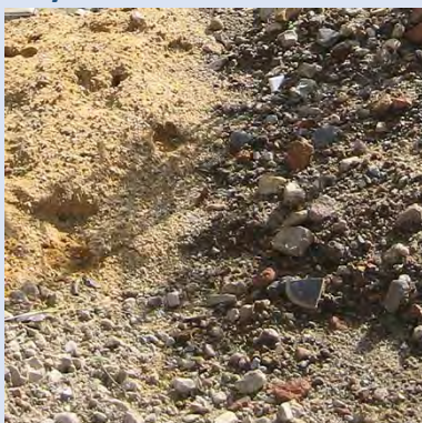
Variety of recycled mineral aggregates used as growing media with depths 100mm to 500mm
